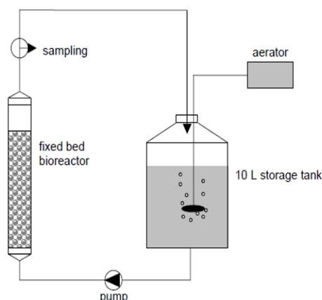
Figure 1. Schematic setup of the FBBR
